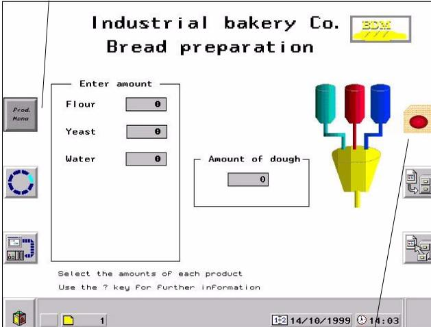
Access to the baking monitoring screen by pressing the R6 dynamic key associated with the icon.
