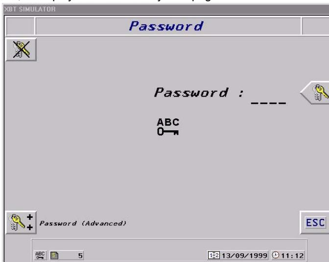
Press the dynamic key associated with the Password icon or press the corresponding touch zone on touchscreen terminals.
