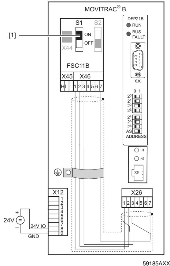
[1] Terminating resistor activated, S1 = ON
