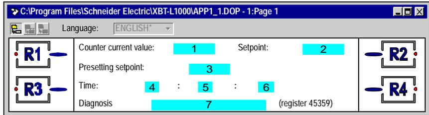
**Field 1** Display counter current value from master (Concept register 401003)
