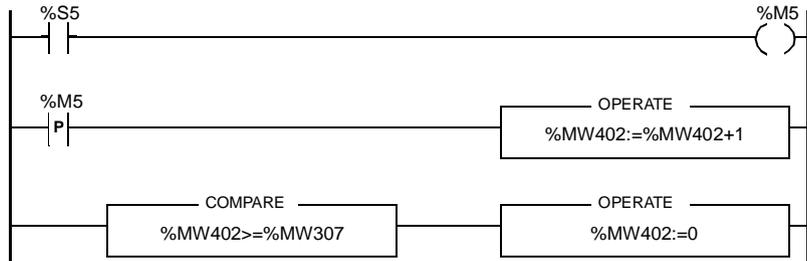
**%MW307** 1st word HMI to PLC table (counter setpoint)
