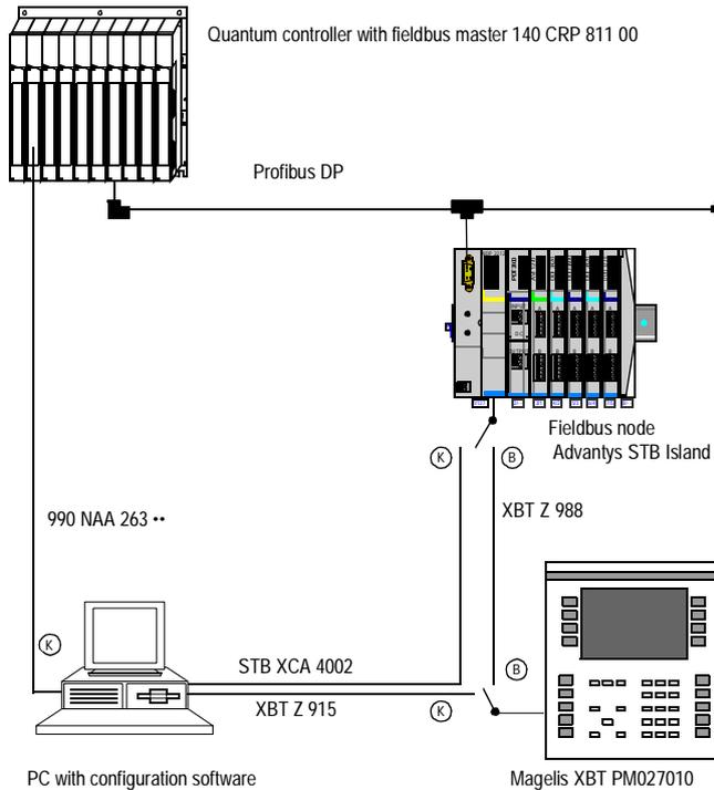
**K** Connections for the transfer of the configurations and programs
