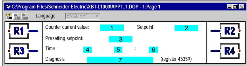
**Field 1** Display counter current value from master (Concept register 401000)
