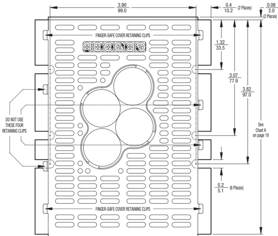
**FIGURE 3B – MODELS KBVF-14, 24, 24D, 26D MECHANICAL SPECIFICATIONS (INCHES/MM)**
