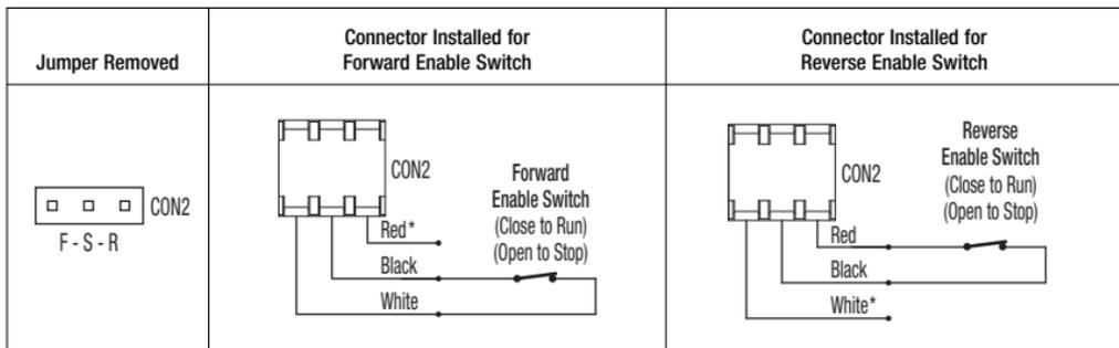
*\*For Forward Enable Switch connection, the red wire is not used. For Reverse Enable Switch connection, the white wire is not used. The unused wire must be insulated or it may be cut off at the connector.*
