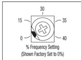
**FIGURE 23 – MAXIMUM SPEED TRIMPOT (MAX) RANGE**
