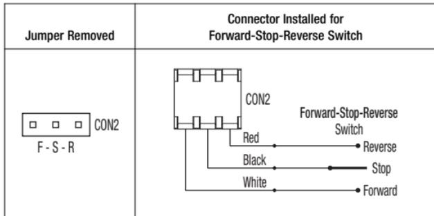
For **Forward Enable Operation**, wire the switch to the white and black wires. For **Reverse Enable Operation**, wire the switch to the red and black wires. When the switch is closed, the drive will run. When the switch is opened, the drive will stop.
