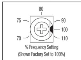
**FIGURE 24 – ACCELERATION TRIMPOT (ACC) RANGE**
