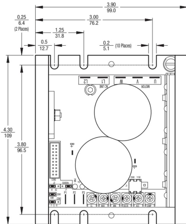
Top View Shown without Finger-Safe Cover Installed
