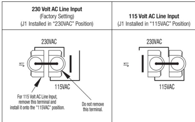
**6.2 60Hz and 50 Hz Motor Operation and Drive Output Frequency Selection (Jumpers J1 and J2)** – Both jumpers must be set for the appropriate motor nameplate frequency rating. Jumpers J1 and J2 are located on the lower PC board.
