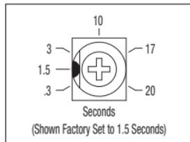
**Application Note** – On applications with high inertial loads, the deceleration may automatically increase in time. This will slow down the rate of speed of decrease to prevent the bus voltage from rising to the Overvoltage Trip point. This function is called Regeneration Protection. **It is recommended that for very high inertial loads that both the ACC and DEC/B Trimpots should be set to greater than 10 seconds.**
