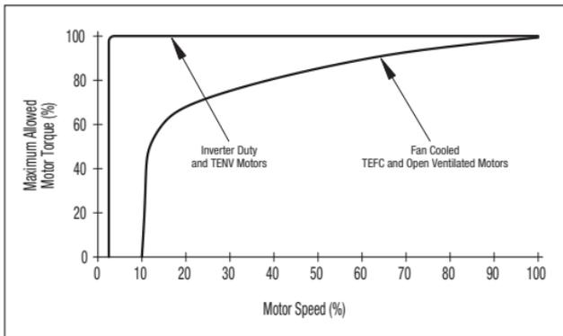
FIGURE 6 – OPEN VENTILATED MOTOR WITH EXTERNAL COOLING
