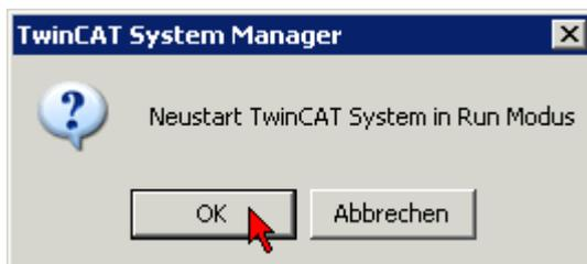
Fig. 160: Restarting TwinCAT in RUN mode
