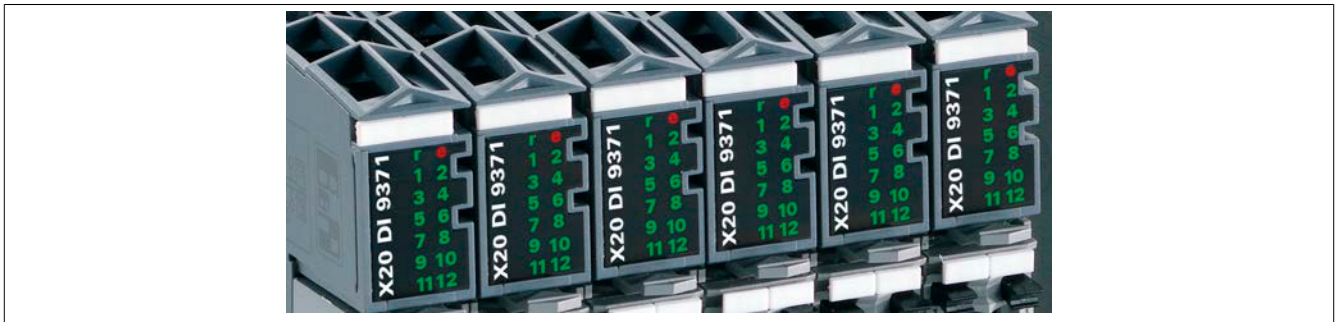
Figure 9: Visual diagnostics directly on the module using LED indicators
