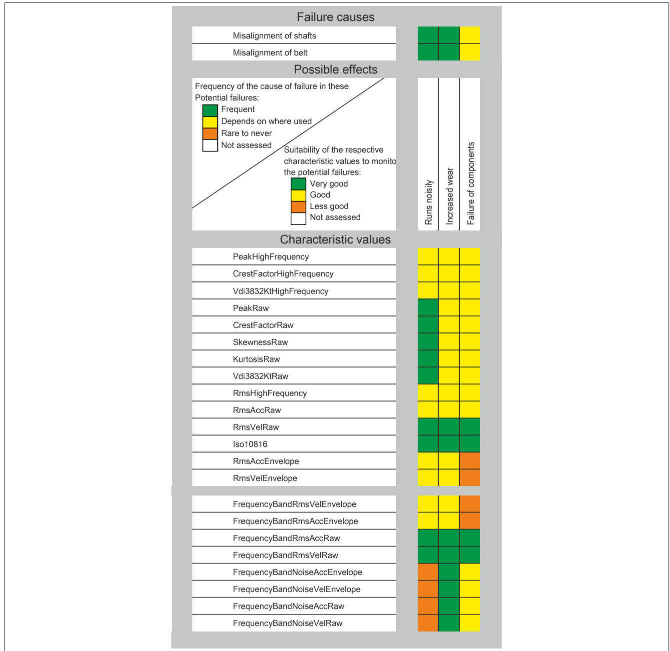
Figure 246: Failure causes and effects of an alignment failure
