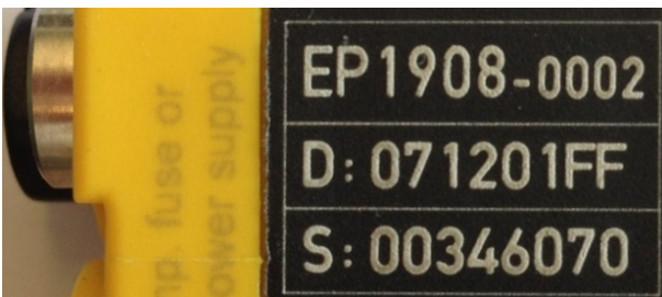
Fig. 6: EP1908-0002 IP76 EtherCAT Safety Box with batch number 071201FF and unique serial number 00346070
