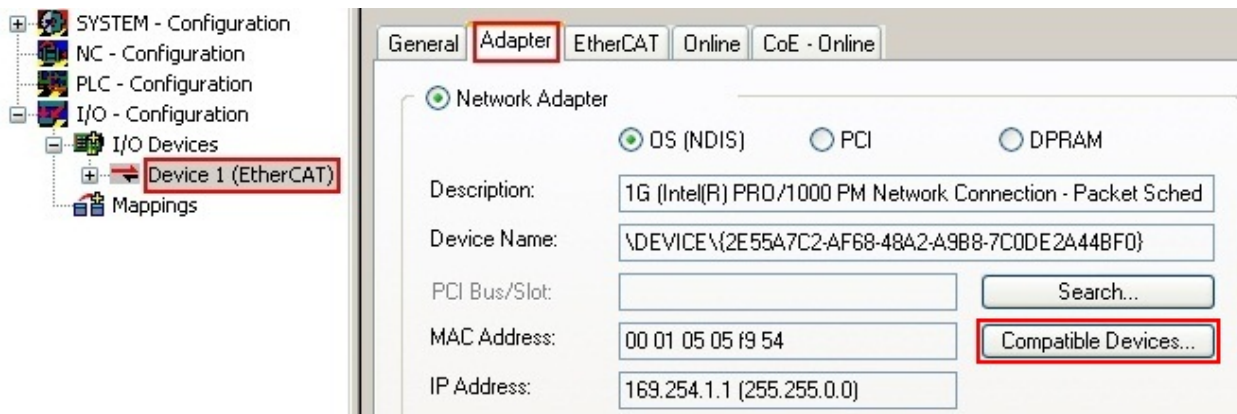
Fig. 35: EtherCAT device properties(TwinCAT 2): click on „Compatible Devices...“ of tab “Adapter”
