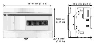
\* 8.5 mm (0.33 in) when the clamp is pulled out.
