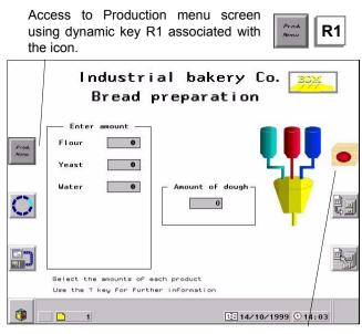
Access to the baking monitoring screen by pressing the R6 dynamic key associated with the icon.
