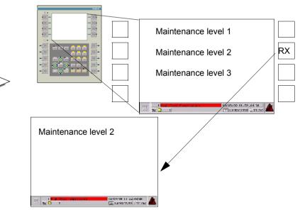
On touchscreen terminals, a page can be selected by directly pressing on a touch zone associated with this page. On terminals with tactile keys, a page can be selected by directly pressing a tactile key.
