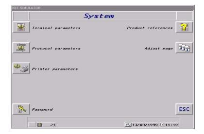
Press the dynamic key (or the touch zone) associated with the Password icon, to display the Password system page.
