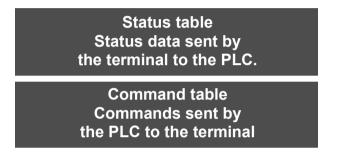
The number of words in the table depends on the choice of status data and commands that are to be processed during the dialog. The XBT-L1000 software allows you to configure the dialog table.
